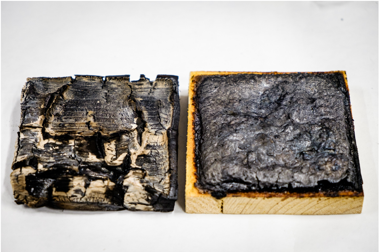
On the left, an example of burnt wood, the right, a piece of wood coated with NTU Singapore's coating (NTU Singapore)
